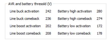
These are read only parameters which varies according to the setting of operation mode and output voltage.
